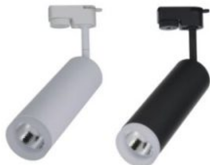
257-D(黑白)-1400 CREE COB 12W 3000K / 4000K 110~240Vac,50/60Hz Beam Angle: 24° Dim.: \varnothing 55 \times 65 \times 185 mm (H)
