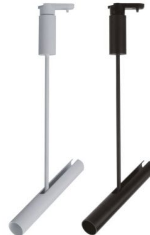
258-D(黑白)-2800 CREE COB 8W 3000K / 4000K 110~240Vac,50/60Hz Beam Angle: 24° Dim.: \varnothing 40 \times 80 \times 440-540 mm(H)
