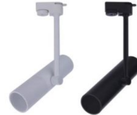
258-B(黑白)-1700 CREE COB 12W 3000K / 4000K 110~240Vac,50/60Hz Beam Angle: 24° Dim.: \varnothing 55 \times 65 \times 210-285 mm(H)
