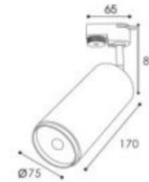
257-E(黑白)-1700 CREE COB 15W 3000K / 4000K 110~240Vac,50/60Hz Beam Angle: 24° Dim.: \varnothing 75 \times 65 \times 170 mm (H)
