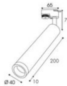
257-B(黑白)-1800 CREE COB 8W 3000K / 4000K 110~240Vac,50/60Hz Beam Angle: 24° Dim.: \varnothing 40 \times 65 \times 210 mm (H)
