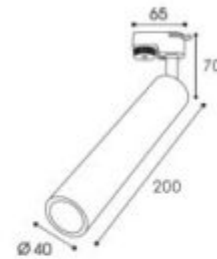
257-A(黑白)-1500 CREE COB 8W 3000K / 4000K 110~240Vac,50/60Hz Beam Angle: 24° Dim.: \varnothing 40 \times 65 \times 200 mm (H)
