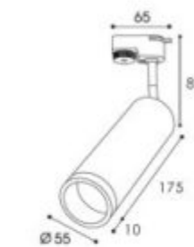
257-D(黑白)-1400 CREE COB 12W 3000K / 4000K 110~240Vac,50/60Hz Beam Angle: 24° Dim.: \varnothing 55 \times 65 \times 185 mm (H)
